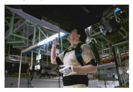
While exoskeletons have been trialled at other car factories, the initiative at Ford's facility in Valencia, Spain, where Galaxy, Kuga, Mondeo, S-MAX and Transit Connect are built, is the first to fully integrate the technology into its production process.
